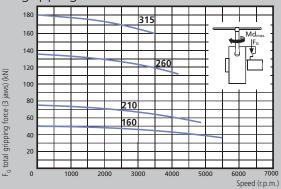
■ The max. gripping force is the total, acting on the 3 jaws, obtained by applying to the chuck the max. allowed driving torque. The data refers to a chuck newly maintained accordingly to their service manual, using SMW K05 grease.
