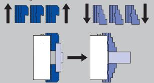
Universal, because jaws can be radially adjusted and reversed = less jaw sets
