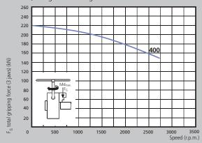
■ The dynamic gripping forces have been measured using hardened standard stepped monoblock jaws type GST placed in a position not exceeding the outer diameter of the chuck.
